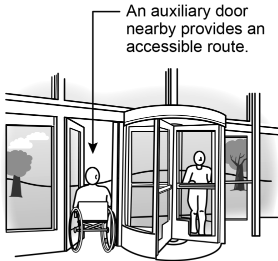
Auxiliary Door at Inaccessible Revolving Door
